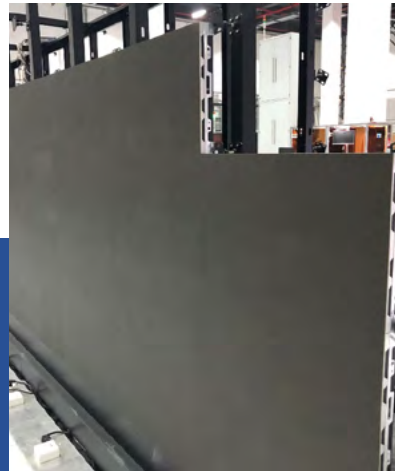
Integration of power and signal cables means no external cables
